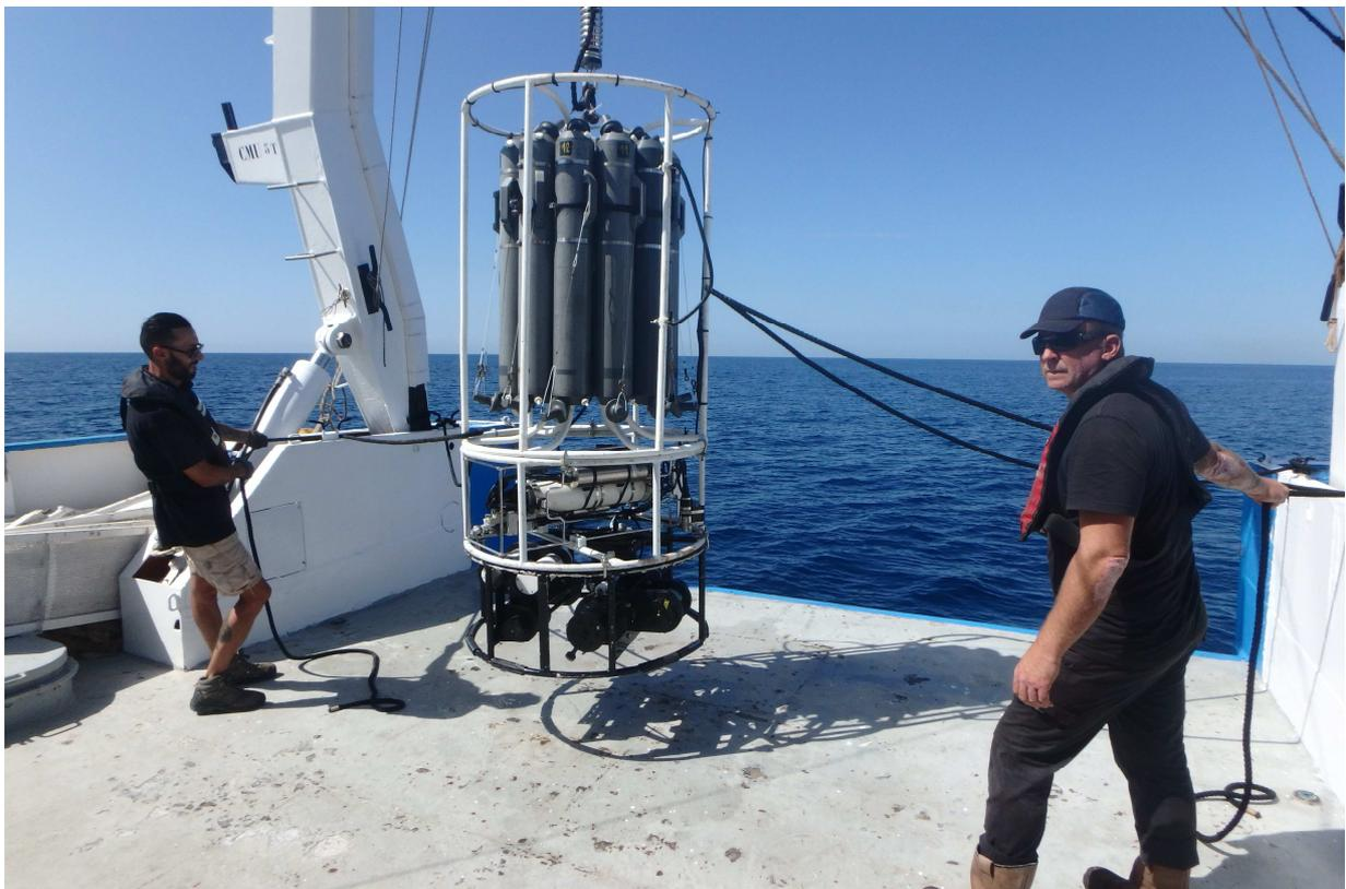
Deployment of the CTD Rosette with IOP package at the BOUSSOLE site.
